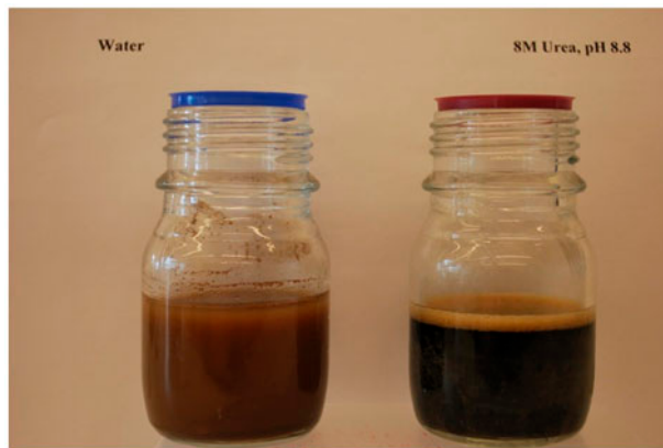
Figure 3. Lignin dispersed in water (left) and dissolved in 8 M urea (right).
